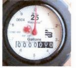
The small red triangle or circle to the left of the needle on the meter face is the low flow indicator. That indicator will spin if any water is flowing through the meter, so it can be useful in leak detection.
